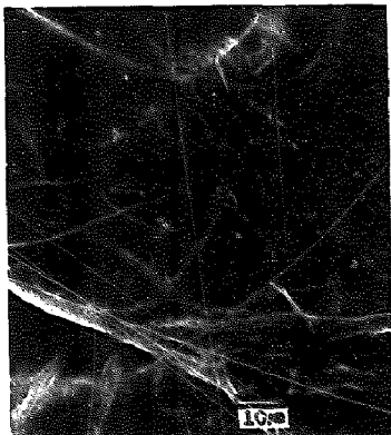
Fig. 1. SEM micrograph of CX-1EC separator, fabricated by matting cellulosic fibres (average diameter \sim 5 \mu\text{m} ) and embedding mat in cellulosic film followed by impregnation with ethylene carbonate.
